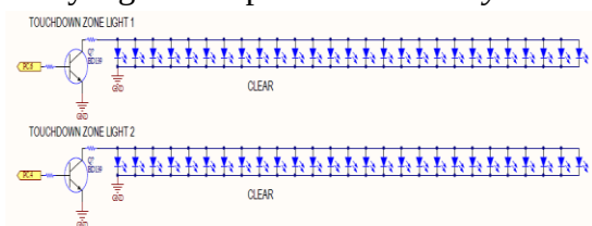
Gambar 42. Wiring Touchdown Zone Light
